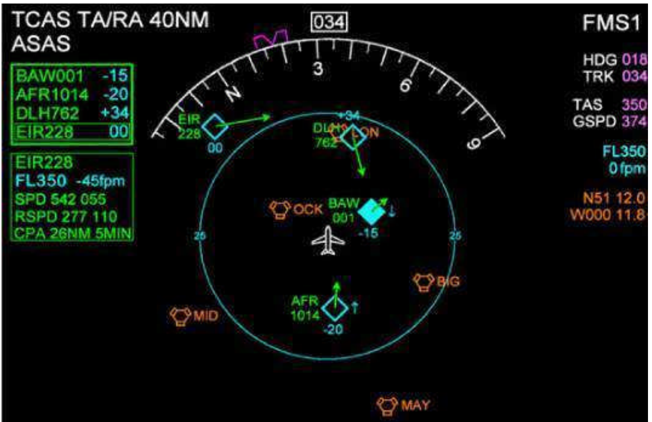
Figure 40c – Type of Navigation Display Showing Information of Other Aircraft Similar to the ND used by UPS crews to maintain spacing behind the lead aircraft during descent and approach, thus making fuel efficient and quiet Continuous Descent Approaches from Cruise Altitude.
