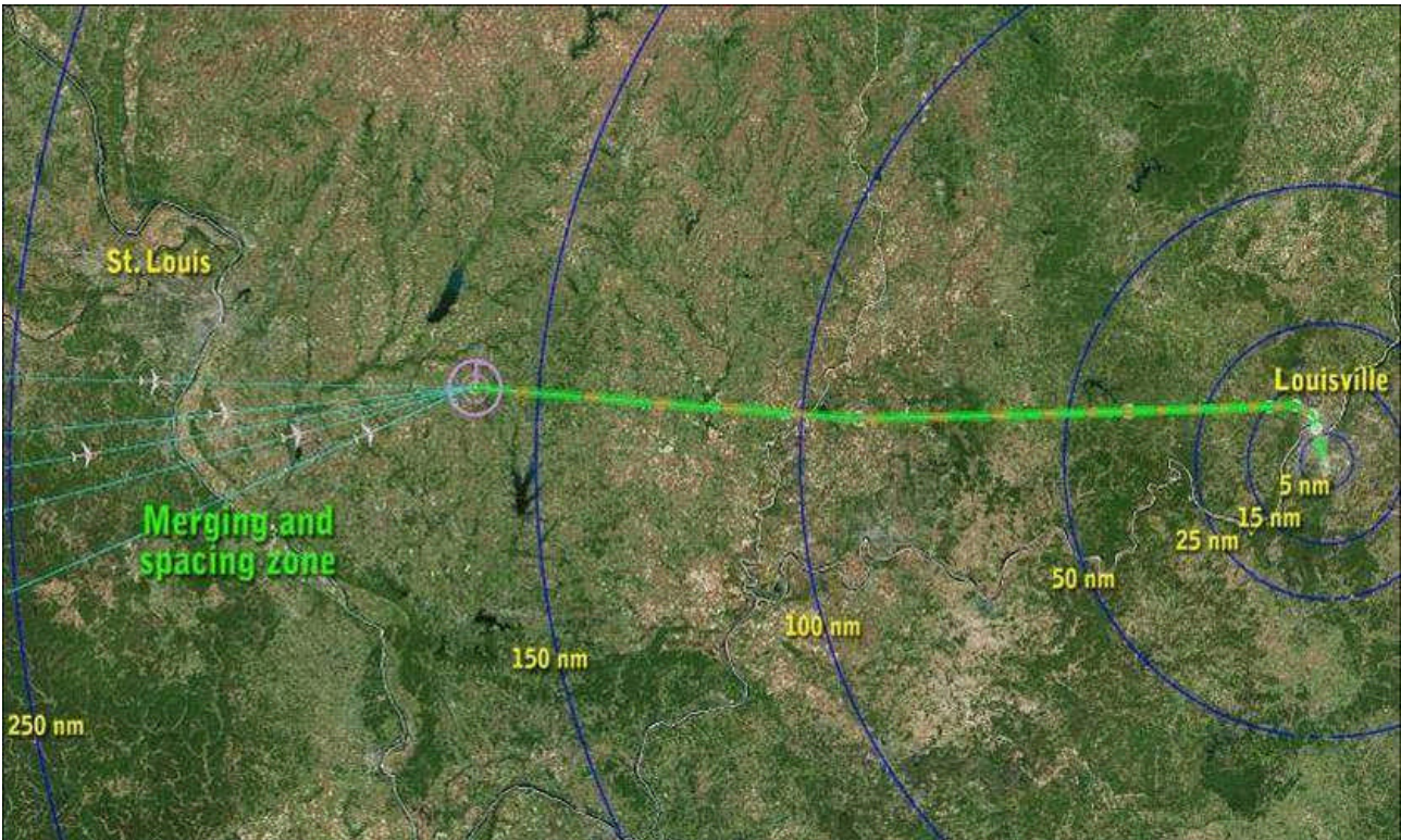
Figure 40a – Satellite image showing the Merging and Spacing Zone in cruise when UPS use their ABESS (Airline Based En-Route Sequencing and Spacing) system to organise their aircraft into an orderly stream prior to descent, when the crews then maintain their spacing from the aircraft they have been told to remain behind using the information on their modified Navigation Displays as in Figure 33b.
