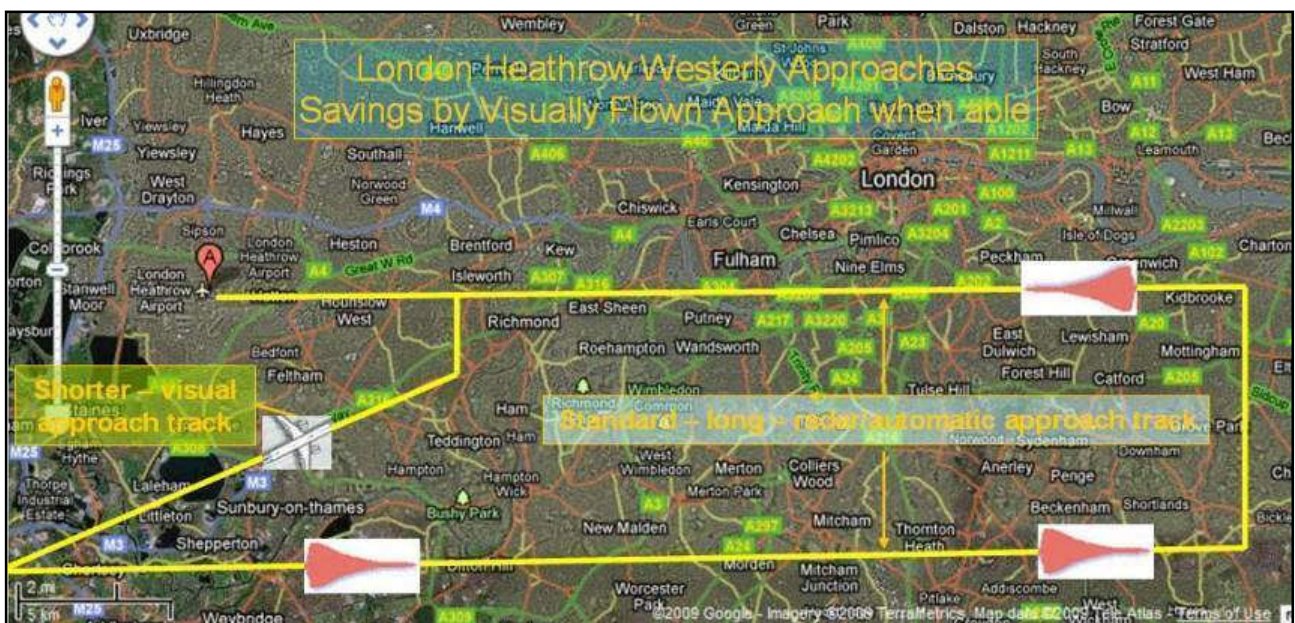
Figure 28 - Ability to Fly a Visual Approach when able to Save Time and Fuel
