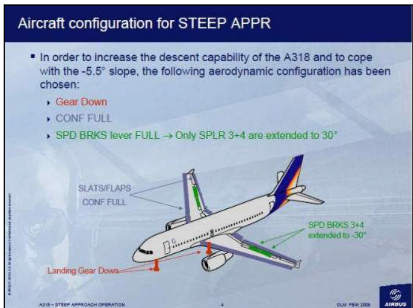
Figure 27 - Airbus A318 Modification for Steep 5.5° Approach For steep approaches on A318s a selection is made to raise spoilers for extra drag and to give early aural warning of the time to flare.
