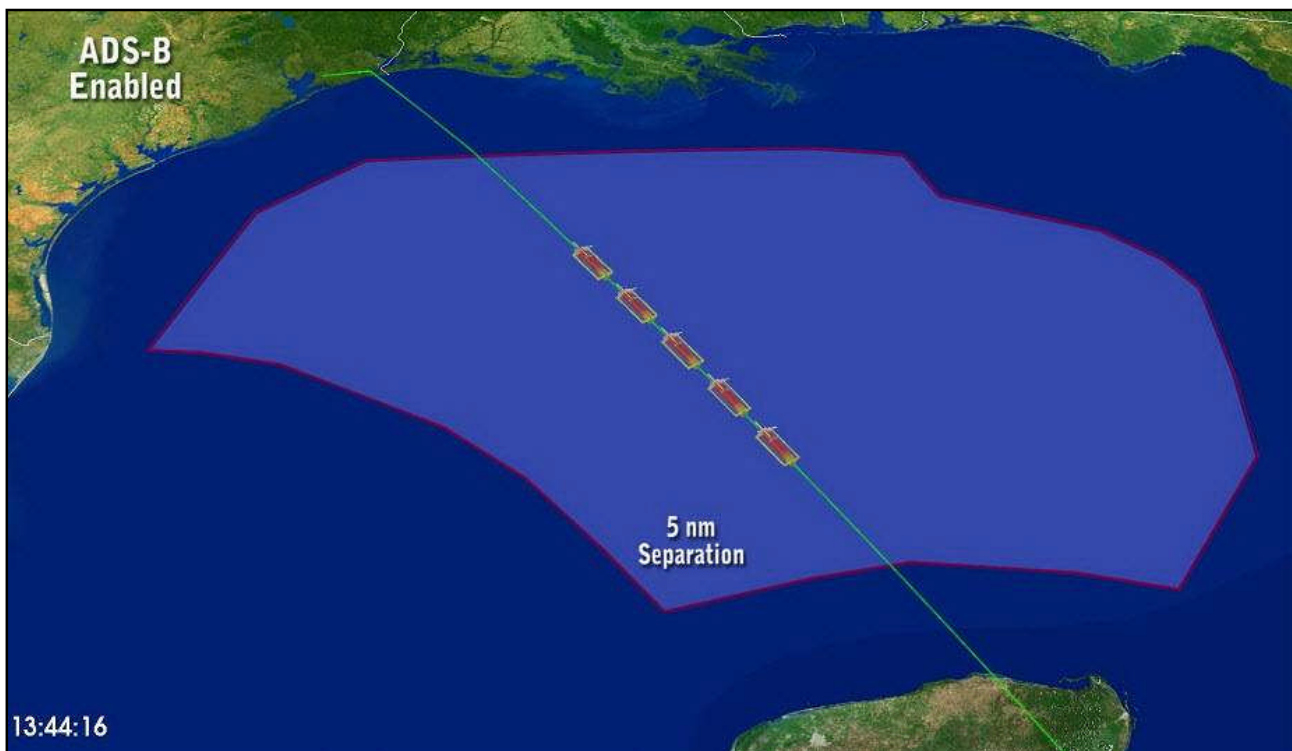
Figure 13b – With ADS-B Enabled, Separation Between Aircraft can be Reduced to 5 nm
