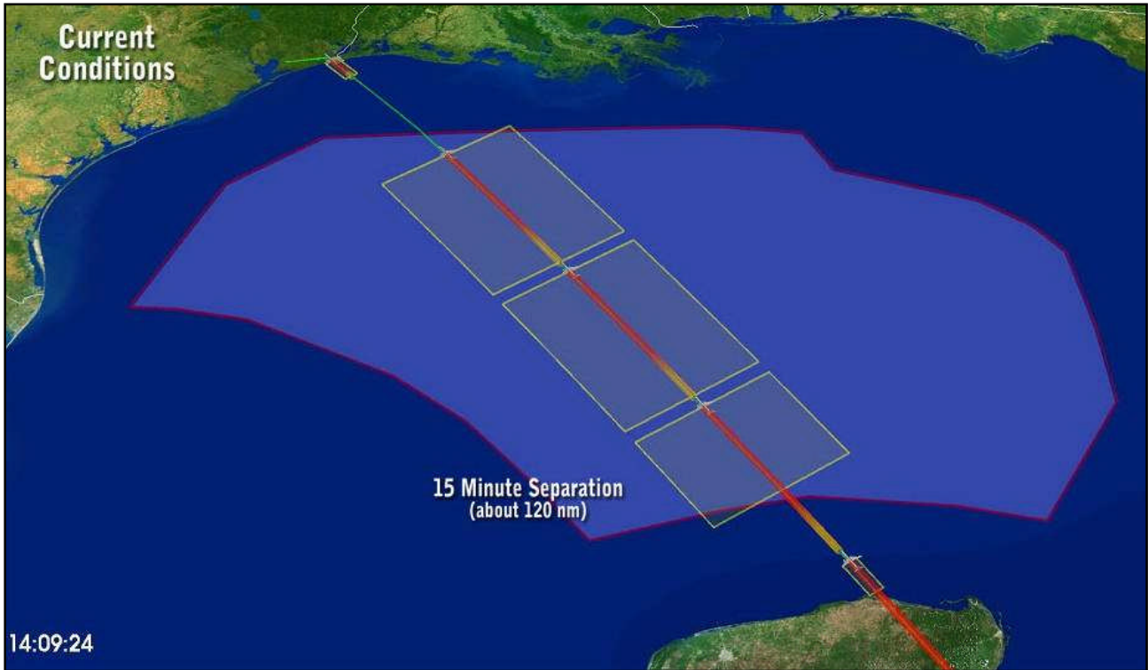
Figure 13a – Current Separation is 15 minute (about 120 n miles) Between Aircraft
