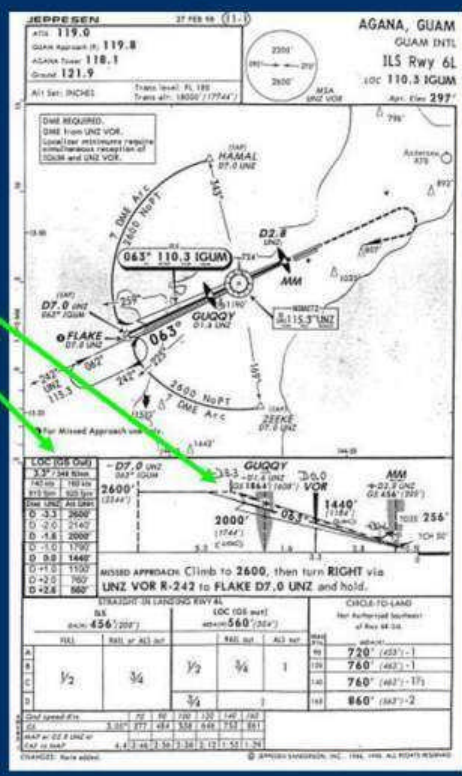
Figure 44 - Second Example of an accident which need not have happened If a the approach had been drawn as a CDA using a DME-Altitude table as shown
