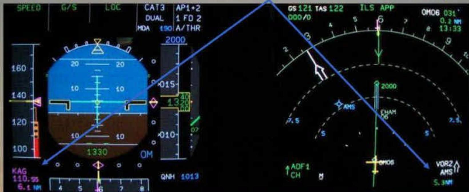
A DME in line with a runway can show an accurate glidepath on a Non Precision Approach by a simple DME-Altitude table for a Constant Descent Angle approach. Many Step Down NPAs accidents could have been avoided over the past 30 years.
