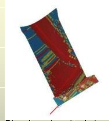
Ply orientation simulation for aerofoil Source: Snecma
