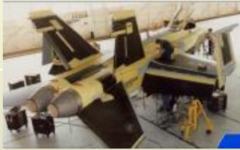
Boeing F18: Carbon composite wing centre box, tail fins and elevators. EIS 1983
